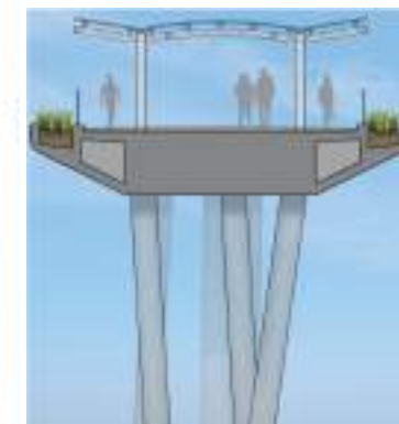
擬建LW-02高架行人道典型橫切面 PROPOSED ELEVATED WALKWAY LW-02 TYPICAL SECTION
