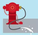
When water supply resumes from a period of suspension, the sediments inside water mains may be stirred up, resulting in slightly higher turbidity in water. The Water Supplies Department (WSD) would drain away the water through fire hydrants until its clarity resumes normal.
