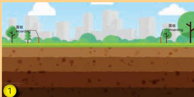
建造工程開始前，先整理工地現場及以圍板圍封工地 Tidy up and fence off the site by hoarding before commencement of construction
